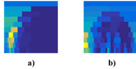
Fig. 6. Sample faulty (a) and healthy (b) signals from vibration signals of metro wheelsets on Kurtogram
